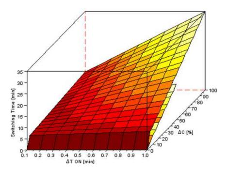
Capacity differences and  $\Delta T$  determine the switching times.
